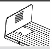
Optional detachable steel bulkhead, 48" head board w/ center opening
