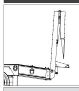
Hydraulic operated apitong covered ramps. BI - FOLD, Self Contained.
