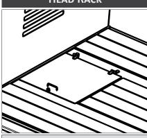
Lockable Tool Box located on top of gooseneck.
