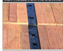
Double slotted key holes gives you more tie-down angles for securing load.
