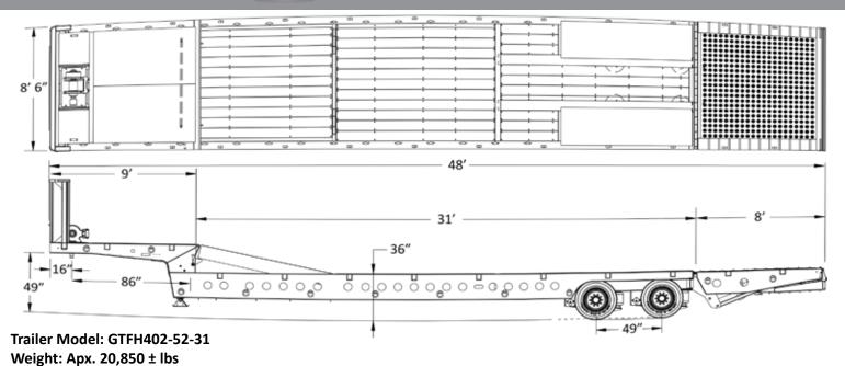
**Overall** Load well 5th Wheel **Hydraulic** Flip Under **Overall** Gooseneck Load well **Swing** Width Length Length Length Height Clearance Tail Ramp Height 48' 8' 6" 9' 31' 36" (Loaded) 86" 49" 8' 4′
