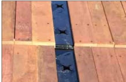
Double slotted key holes gives you more tie-down angles for securing load.
