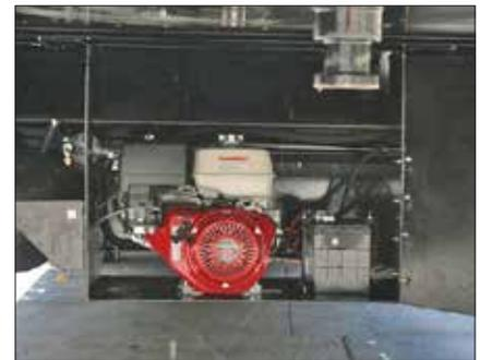
Gasoline 10, 11 or 13 Horse Power Pony provides the hydraulic operation of the tail. Self-contained under the neck.
