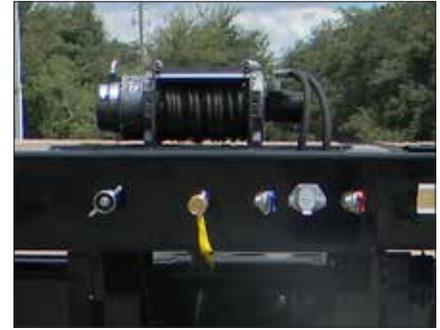
Available options for 12,000 to 30,000 lb hydraulic winch system. Mounted front and center of the upper deck. Standard cable length of 85' with shackle. Cable length options are available.
