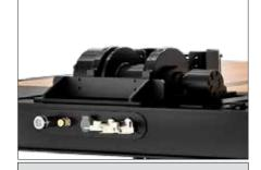
Available options for 12,000 to 30,000 lb hydraulic winch system. Mounted front and center of the upper deck. Standard cable length of 85' with shackle. Cable length options are available.
