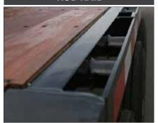
2 ½" rolled formed steel. 6" Structural Channel @ 6.5 lbs/ft, 5/16" Thick Stake Pockets 1 5/8" x 3 ½" x ¼", 24" O/C, ¼" x 3" Rub rail.
