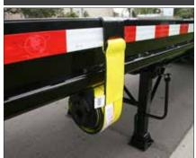
Web winches can be located on either side. Used to secure loads and objects on the trailer.
