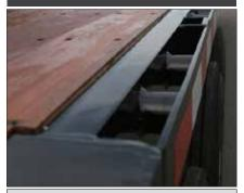
$2 \frac{1}{2}$ " rolled formed steel. 6" Structural Channel @ 6.5 lbs/ft, 5/16"Thick Stake Pockets 1 5/8" x 3  $\frac{1}{2}$ " x  $\frac{1}{4}$ ", 24" O/C,  $\frac{1}{4}$ " x 3" Rub rail.
