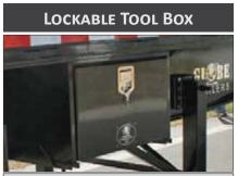
Optional Lockable Tool Box Mounted Underside of Main Deck, 24" x 24" x 48" Steel, can be located on either side.
