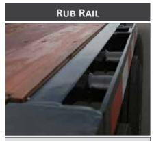
2 1/2" rolled formed steel. 6" Structural Channel @ 6.5 lbs/ft, 5/16" Thick Stake Pockets 1 5/8" x 3 1/2" x 1/4", 24" O/C, 1/4" x 3" Rub rail.
