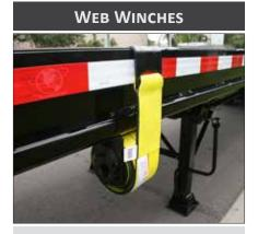
Web winches can be located on either side. Used to secure loads and objects on the trailer.
