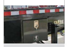
Optional Lockable Tool Box Mounted Underside of Main Deck, 24" x 24" x 48" Steel, can be located on either side.
