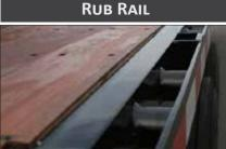
2 <sup>1</sup>/<sub>2</sub>" rolled formed steel. 6" Structural Channel @ 6.5 lbs/ft, 5/16" Thick Stake Pockets 1 5/8" x 3 1/2" x 1/4", 24" O/C, 1/4" x 3" Rub rail.
