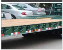
Equipped with outriggers to help support the extra wide loads.
