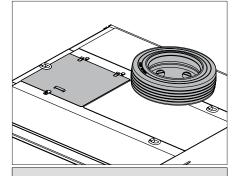
Tool box & Spare tire are located on the front section of the upper deck.
