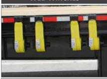
Web winches are welded on, located on the road side. Used to retain loads and objects on the trailer.
