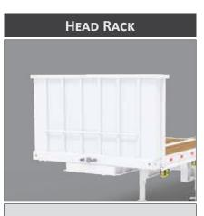
Optional detachable steel bulkhead, with chain rack.
