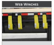
Web winches are welded on, located on the road side. Used to retain loads and objects on the trailer.
