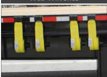
Web winches are welded on, located on the road side. Used to retain loads and objects on the trailer.
