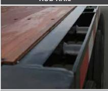
2 ½" rolled formed steel. 6" Structural Channel @ 6.5 lbs/ft, 5/16" Thick Stake Pockets 1 5/8" x 3 ½" x ¼", 24" O/C, ¼" x 3" Rub rail.
