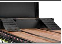
Pull out aluminum ramps built into neck to load wheeled vehicles onto upper deck.
