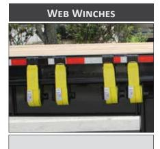
Web winches are welded on, located on the road side. Used to retain loads and objects on the trailer.
