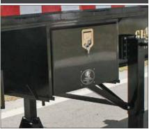
Optional Lockable Tool Box Mounted Underside of Main Deck, 24" x 24" x 48" Steel, can be located on either side.
