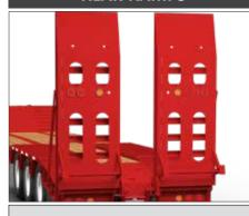
Adjustable with spring assist and safety bar.
