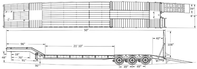
Trailer Model: GTFV403-50-30 Weight: Apx. \_\_\_\_\_ ± lbs
