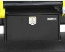
Optional Lockable Tool Box Mounted Underside of Main Deck, 24" x 24" x 48" Steel, curb side.
