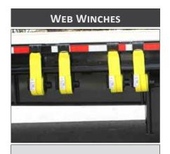
Web winches are welded on, located on the road side. Used to retain loads and objects on the trailer.
