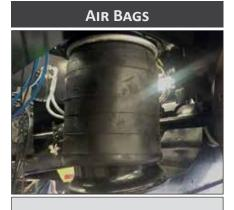
30,000 pound rated large diameter air bags are standard. This allows for lower operating pressure and higher capacity when needed.
