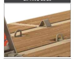
Lifting Lugs for Air Lift.
