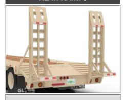
Adjustable with spring assist and safety bar.
