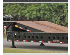
The Hydraulic Ramps extend to allow easier loading on to the upper deck.
