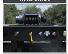
Available options for 12,000 to 30,000 lb hydraulic winch system. Mounted front and center of the upper deck. Standard cable length of 85' with shackle. Cable length options are available.
