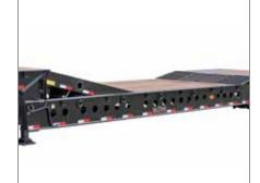
The drop deck design allows for taller loads.
