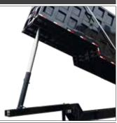
The hydraulic lift cylinder allows and restricts the trailer dumping angle up to 45°, which is optimal for ejecting debris and maintaining a safe operating height.
