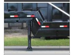
The drop deck allows for more volume and reduces overall height, also the trailer is safer than other trailers due to the lower center of gravity.
