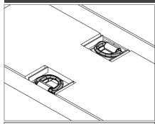
"D" Ring tie downs on lower deck with a design load of 15,000 lbs.
