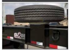
Spare tire mounted on top of the gooseneck
