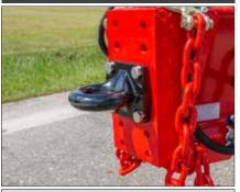
3" Pintle eye, with 4 adjustable height positions, with 2 heavy duty safety chains and grab hooks.
