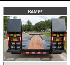
Adjustable with Hydraulic assist and safety bar.
