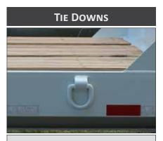
D-rings on each side of the deck make it easier to secure loads to the trailer.
