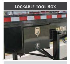
Optional Lockable Tool Box Mounted Underside of Main Deck, 24" x 24" x 48" Steel, can be located on either side.
