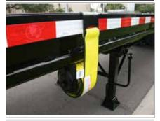
Web winches can be located on either side. Used to secure loads and objects on the trailer.
