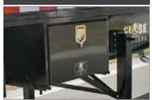
Optional Lockable Tool Box Mounted Underside of Main Deck, 24" x 24" x 48" Steel, can be located on either side.
