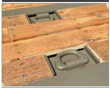
Four (4) lift rings on top of deck for lifting aboard ships.
