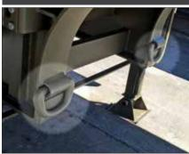
Four (4) tie downs located on underside of trailer for air transportability. In accordance with -IAW MIL-HDBK-1791.
