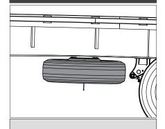
Spare tire wheel assembly with basket carrier under chassis curbside.
