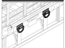
Tie down rings at rear on the bumper, and at front near the landing gear.
