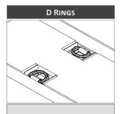
"D" ring tie downs on upper and lower deck with a design load of 15,000 lbs.
