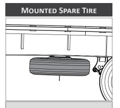
Spare tire wheel assembly with basket carrier under chassis curbside.
