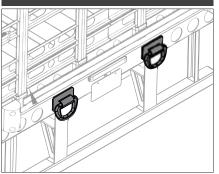
Tie down rings at rear on the bumper, and at front near the landing gear.
