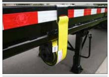
Web winches can be located on either side. Used to secure loads and objects on the trailer.
