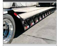
With a standard deck height of 18", Globe Trailers have lower overall height, which allows taller loads to be hauled.
