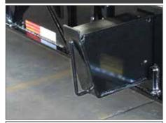
Globe Trailers fabricated heavy duty pullout front outriggers provide added strength which is needed to accommodate the initial force when loading equipment. The outrigger is held in position with a spring loaded locking pin.
