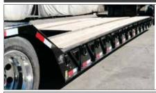
With a standard deck height of 18", Globe Trailers have lower overall height, which allows taller loads to be hauled.
