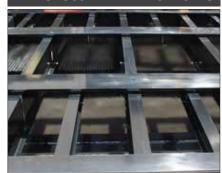
Standard 12" stubbed cross member spacing produces added strength to the trailer and also less stress on the decking, leading to a longer life of the decking material.
