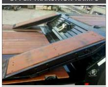
Adjustable sliding transition ramps with wood covering for traction.
