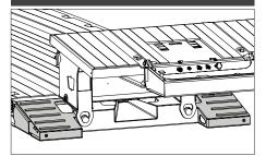
Low profile built-in integrated deck ramps.
