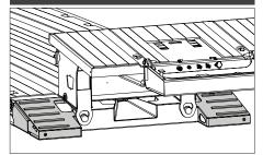
Low profile built-in integrated deck ramps.
