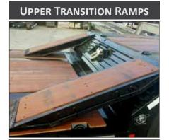
Adjustable sliding transition ramps with wood covering for traction. Ramps are removable.
