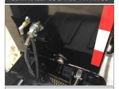
Air, electric and hydraulic (when applicable) fittings are all centrally located at the base of the gooseneck inside a bolster. This makes for quick and easy connect and disconnect.
