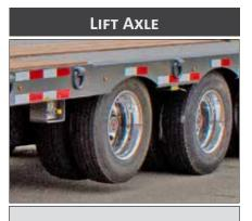
Lift Axle distributes the load carrying capacity on the other axles, also increases the tire & axle life over wear & tear. Keep lifted in unloaded, and grounded in loaded conditions.
