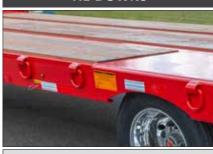
D-rings on each side of the deck make it easier to secure loads to the trailer.
