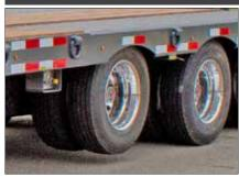
Lift Axle distributes the load carrying capacity on the other axles, also increases the tire & axle life over wear & tear. Keep lifted in unloaded, and grounded in loaded conditions.
