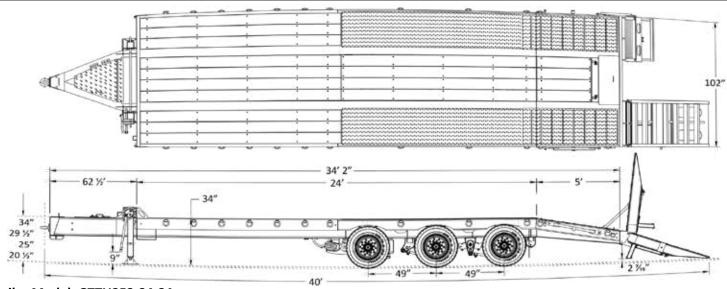
Trailer Model: GTTU253-34-24 Weight: Apx. \_\_\_\_ ± lbs
