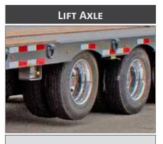
Lift Axle distributes the load carrying capacity on the other axles, also increases the tire & axle life over wear & tear. Keep lifted in unloaded, and grounded in loaded conditions.
