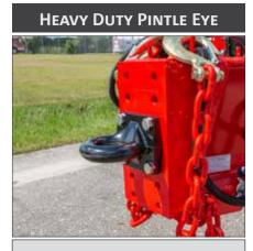
3" Pintle eye, with 4 adjustable height positions, with 2 heavy duty safety chains and grab hooks.
