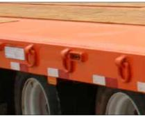
D-rings on each side of the deck make it easier to secure loads to the trailer.
