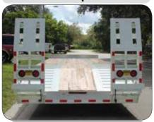
Adjustable with spring assist and safety bar.
