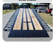
Multiple Deck width setting allow for extending the deck width from 102" to 150".
