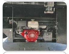
Gasoline 10, 11 or 13 Horse Power Pony provides the hydraulic operation of the tail. Self-contained under the neck.
