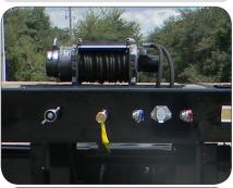
Available options for 12,000 to 30,000 lb hydraulic winch system. Mounted front and center of the upper deck. Standard cable length of 85' with shackle. Cable length options are available.
